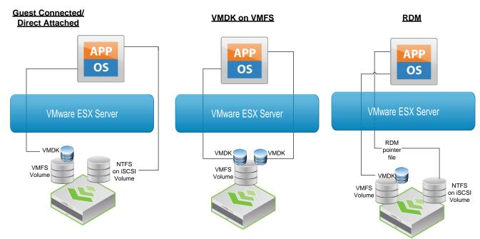
Figure 6: Three types of disk connectivity methods for virtual machines
