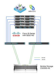
Scalable VDI environment for 300+ users using Nimble Storage hybrid arrays, Cisco UCS, and VMware Horizon View.
