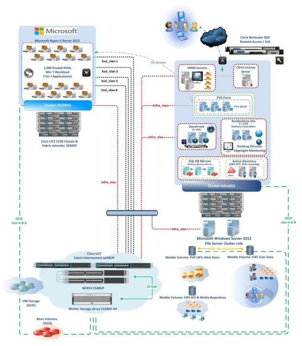
Figure 4. Hosted Virtual Desktops - Logical Component View
