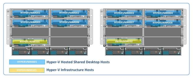
Figure 10. Hyper-V Host to Chassis Assignment for HSDs
