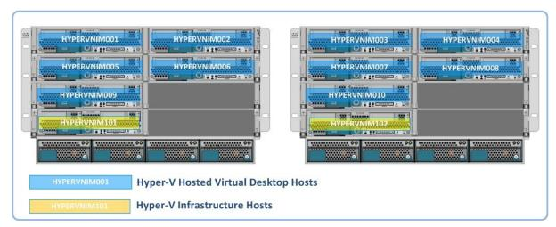
Figure 11. Hyper-V Host to Chassis Assignment for HVDs
