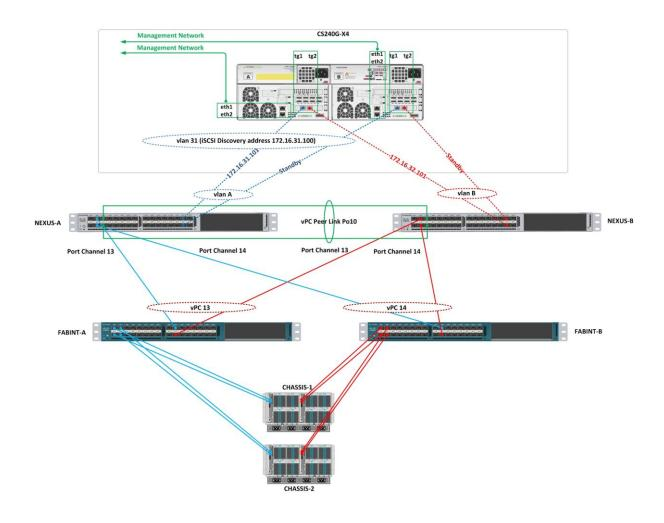
Figure 7. Network Component Connectivity
