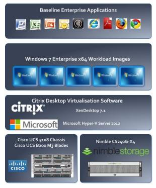
Figure 2. Solution Stack HVD Workload
