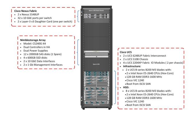
Figure 5. Physical Component View HSD
