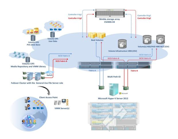
*Figure 8.* below provides a high level overview of the Nimble Storage architecture and describes a typical Hyper-V Host.
