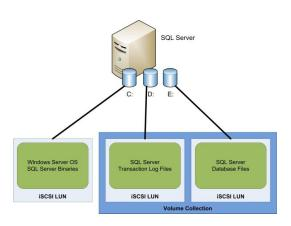
database and transaction logs on different volumes. For example, transaction logs have heavy sequential write activity while database files have more random read/write activity.
