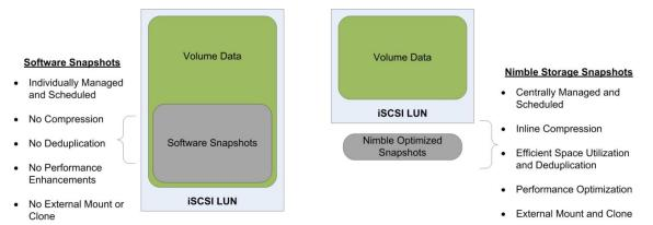
Beginning with SQL Server 2005 Enterprise, SQL Server also contains snapshot features that require SQL scripting skills. These types of SQL Server application-native snapshots are stored within the database files and use copy-on-write methodology that is very inefficient when compared with Nimble Storage array snapshot backups. Using Nimble Storage arrays, Database Administrators can perform database snapshots much more frequently and with more granular recovery points. These maintain the
