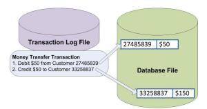
customer. When SQL Server tells the operating system to write the transaction, it also tells it to make sure that no hardware caches the write in memory and that it goes directly to a disk. After the transaction log write completes, SQL Server can update the database file to reflect the new first customer balance of \$50 and then update the database file to \$150 for the second customer.
